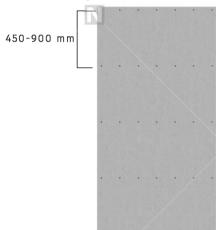
2 According to pre-drilled hole, use expansion screw to fix U shape fastener to the concrete wall.
