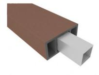
Pre-drill galvanized square pipe and WPC louver tube at the same time, distance of pre-drill hole should be same distance as pre-drilled hole on wall.
