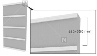
Pre-drill metal joist horizontally according to needed distance.
