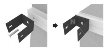
Insert galvanized square pipe into WPC louver tube, galvanized square pipe should be same length as WPC louver tube.
