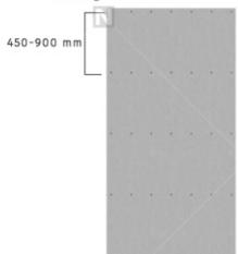
According to pre-drilled hole, use expansion screw to fix U shape fastener to the concrete wall.
